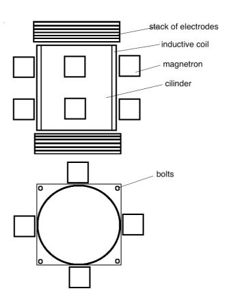
The output energy at the stack of electrodes, could be of direct current, thus we should implement some standard converters, to convert it to alternating current and to add it to the electrical power network.
