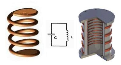
The both resonant circuits should be harmonically adjusted to each another therefore some outer regulated inductor could be used to match the resonance with inner LC circuit. The frequency of pulsed high voltage power supply should also harmonically match the resonant frequency of coupled resonant circuits. In doing so, the decontamination process could even be accelerated thus the electric power converted by absorbers could be higher.
